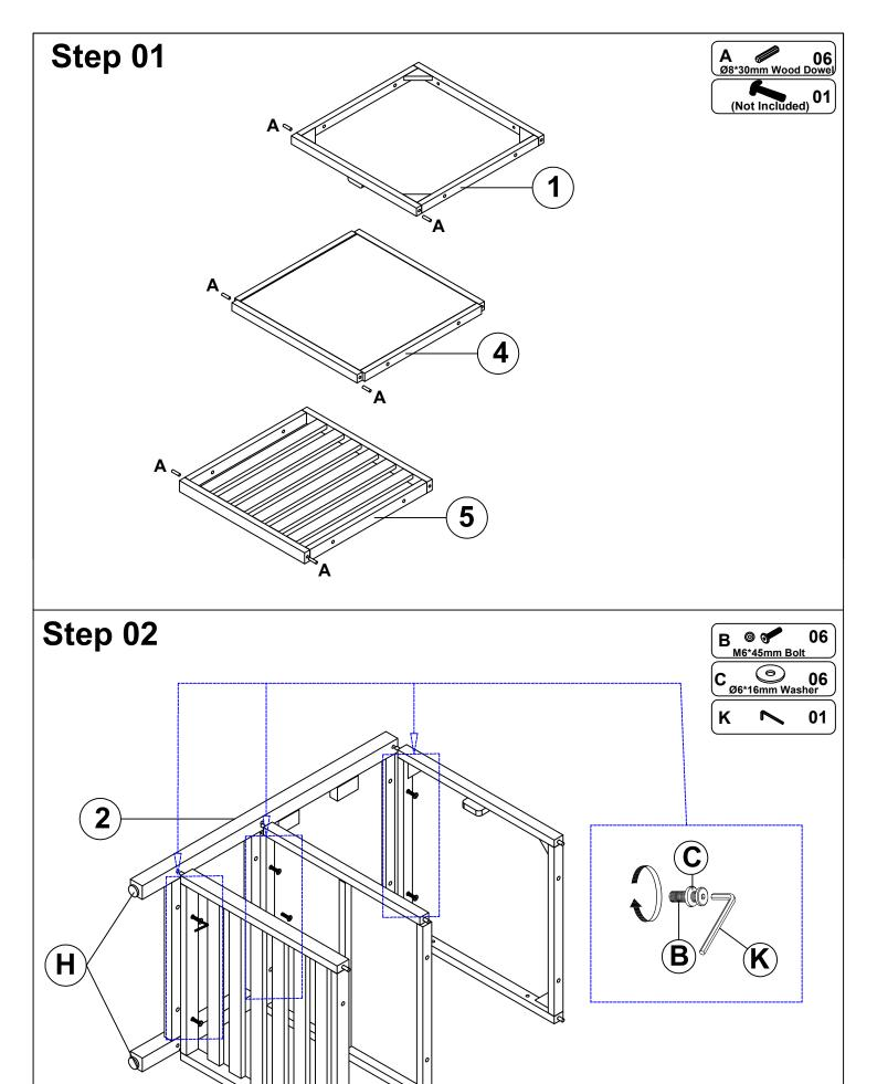
Note: Do not tighten bolts firmly at this time
