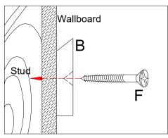
Step 7: If hole locations do not align with stud in wall, install the EZ Anchor(G) in to drywall by tapping it in to the predrilled pilot holes up to the thread, and then screwing the EZ Anchor in to the drywall. Attach Cleat (B) using wood screw (F) to EZ Anchors. NOTE: Cleat could be secured using combination of Studs and EZ Anchors.
