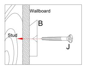
Step 8: If hole locations do not align with stud in wall, install the EZ Anchor(K) in to drywall by tapping it in to the predrilled pilot holes up to the thread, and then screwing the EZ Anchor in to the drywall. Attach Cleat (B) using wood screw (J) to EZ Anchors. NOTE: Cleat could be secured using combination of Studs and EZ Anchors.
