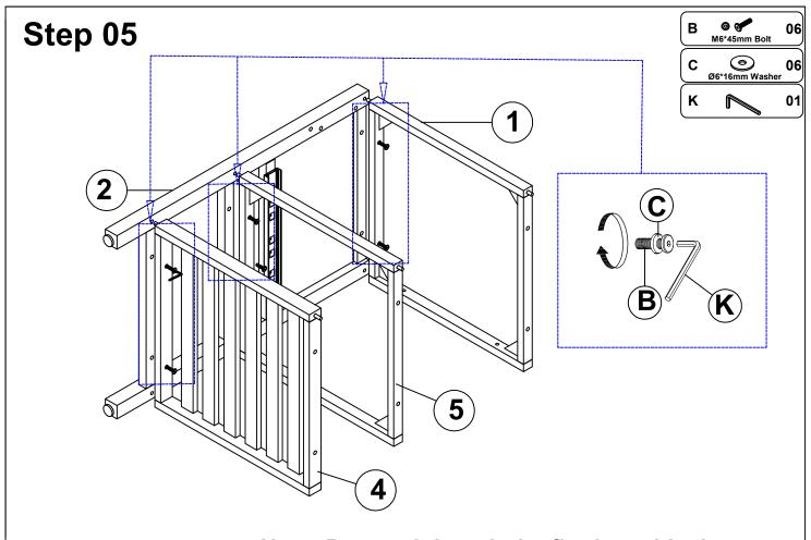
Note: Do not tighten bolts firmly at this time
