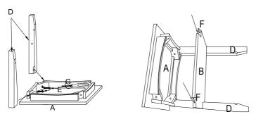
**Step 4** Attach Bottom (C) using 2 Hex Bolts 45mm (E). Repeat same procedure with other 2 Posts (D).
